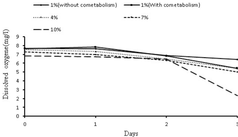
**Figure 5:** This figure shows the amount of dissolved oxygen at the concentrations of 1, 4, 7, and 10 percent of hexadecane and concentration of 1 percent of hexadecane along with co-metabolism in the main SSBR.
