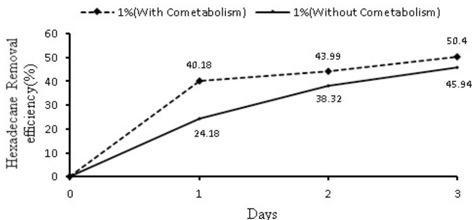
**Figure 6:** This figure shows the comparison of the removal percentage of hexadecane at the concentration of 1% hexadecane in two conditions with and without co-metabolism (glucose) in the SSBR.
