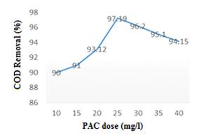
Figure 2: Effect of coagulant along with clarifier sludge on COD Removal
