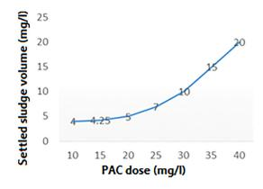
Figure 4: The effect of the coagulant with the clarifier sludge on settled sludge volume
