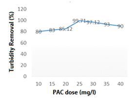
Figure 1: Effect of coagulant with clarifying sludge on Turbidity Removal
