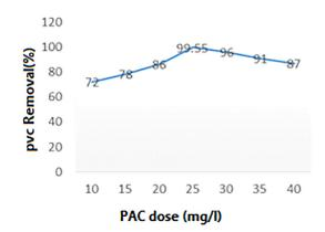
Figure 3: The effect of coagulant along with the clarifier sludge on PVC removal (%)
