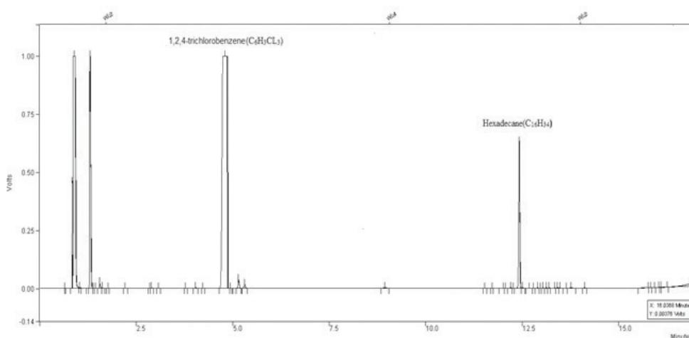
**Figure 7:** This figure shows the GC-FID chromatogram of hexadecane and 1, 2, 4-trichlorobenzene.
