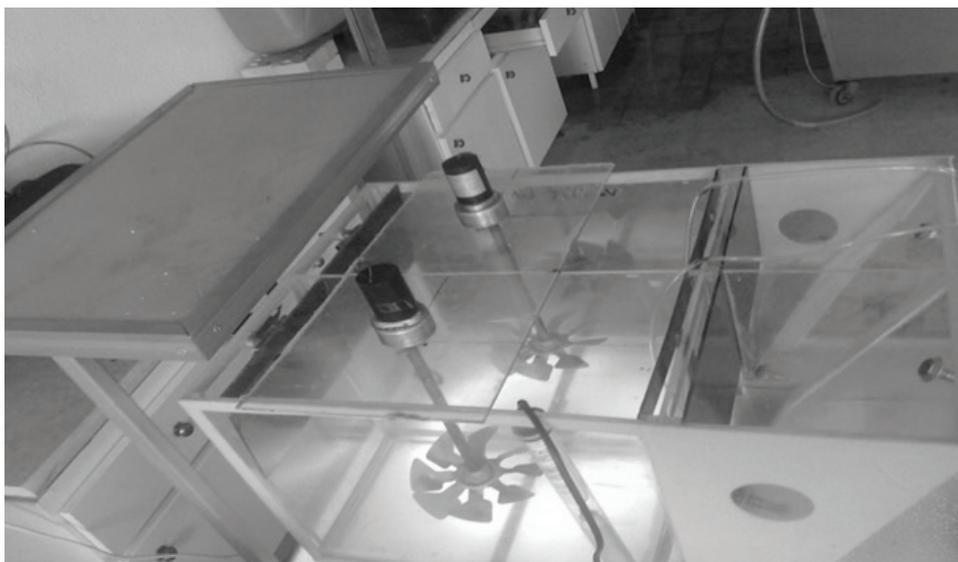
**Figure 1:** This figure shows the Slurry Sequencing Batch Reactor (SSBR).
