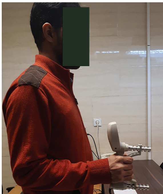
Figure 2: A subject while exerting force to JHD (force exerted in neutral wrist/hand posture)
