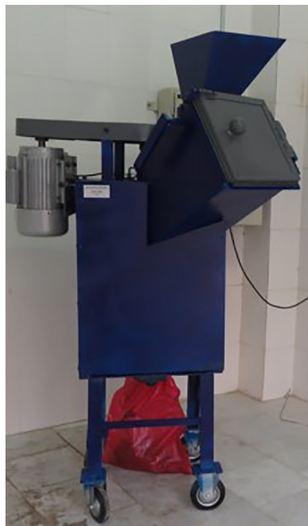
Figure 1: Designed and constructed decontamination device for hospital waste by chemical and mechanical methods
